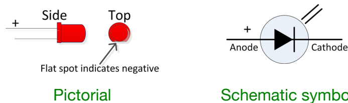
Figure 4-2. LED shown in pictorial and schematic forms
