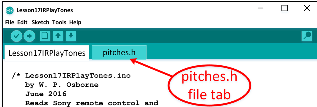
Figure 17-3. Portion of Arduino™ IDE showing tab for pitches.h file
