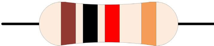
*Figure HT4-3: Resistor (expanded greatly from actual size)*
